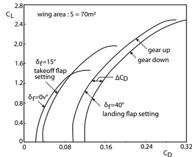
FIGURE 2.11: Typical lift-drag polars for propeller-driven transport airplane (estimated) (Ruijgrok, 2009)
