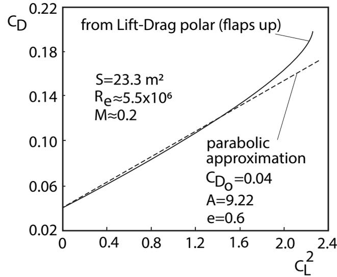
FIGURE 2.14: Parabolic approximation of lift-drag polar of low-subsonic airplane (Ruijgrok, 2009)
