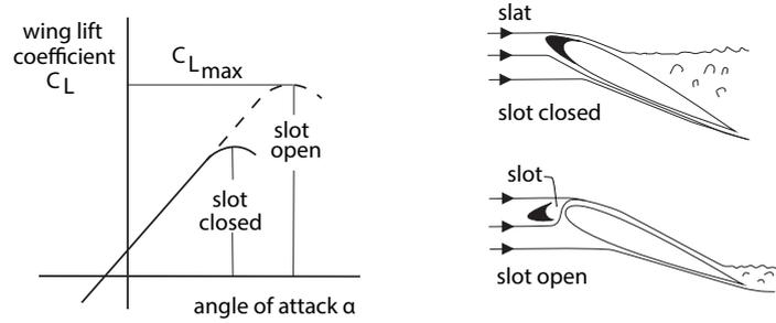
FIGURE 2.8: Effect of a slot on wing lift curve (Ruijgrok, 2009)
