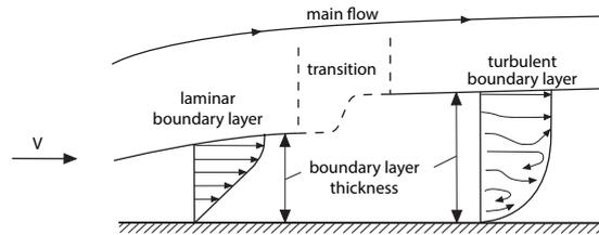
FIGURE 2.12: Typical laminar and turbulent boundary layer velocity profiles (Ruijgrok, 2009)
