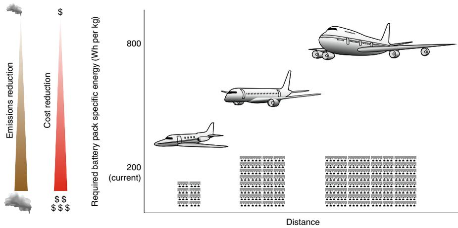
FIGURE 1.5: Electric aircraft scaling (Viswanathan & Knapp, 2019).
