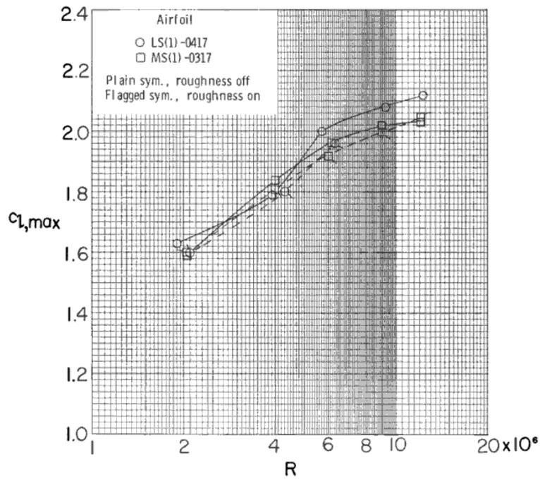
FIGURE 3.4:  $c_{l,max}$  for various Reynolds numbers.
