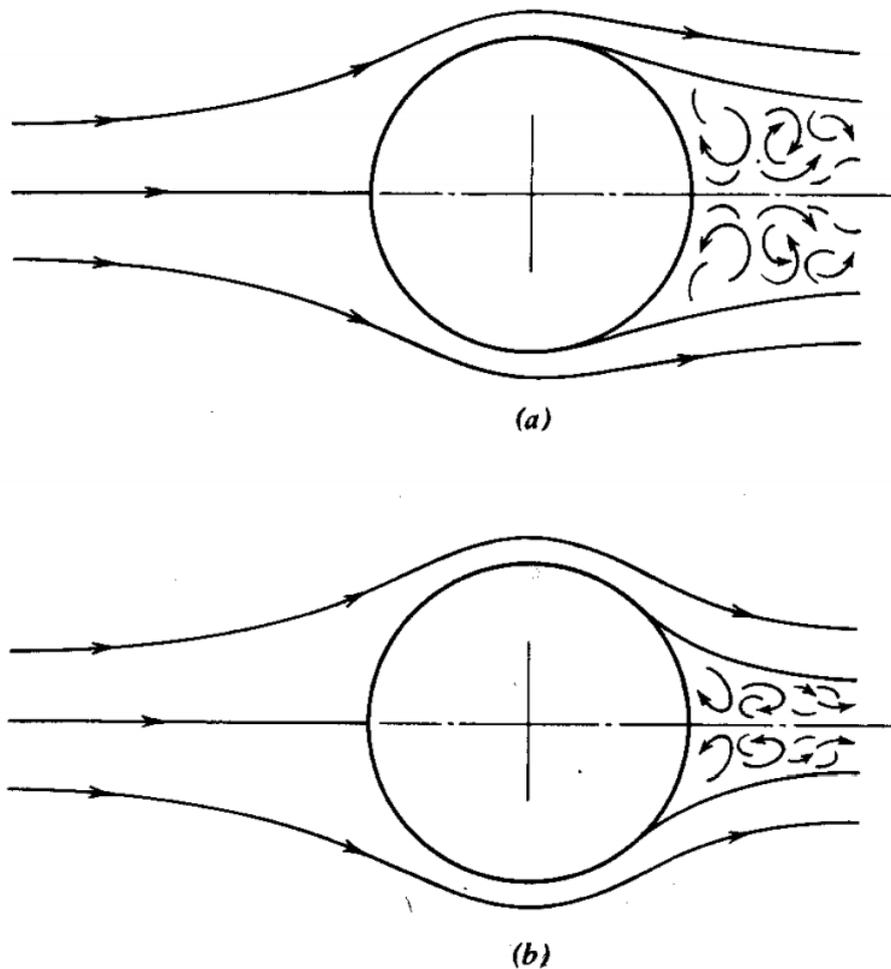
FIGURE 2.18: Flow over a circular cylinder. (a) Low Reynolds number. (b) High Reynolds number. (McCormick, 1994)
