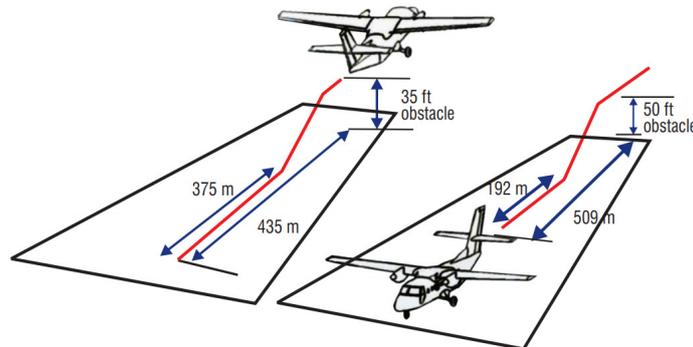
FIGURE 1.7: N-219 Take-Off and Landing illustration (*N219 SOLUTION FOR FRONTIER GATEWAY*, 2018).
