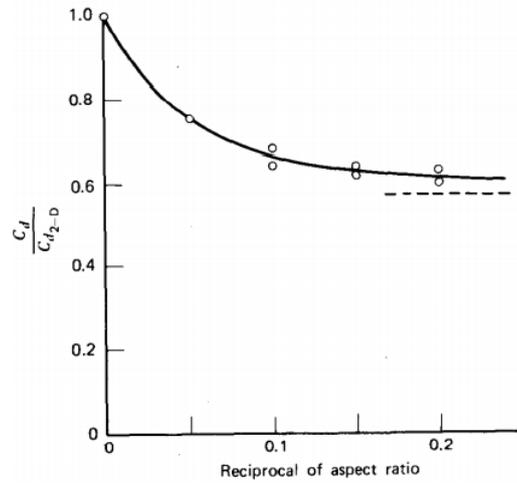
FIGURE 2.21: Transition from three-dimensional to two-dimensional drag for cylinders at supercritical Reynolds number. (McCormick, 1994)
