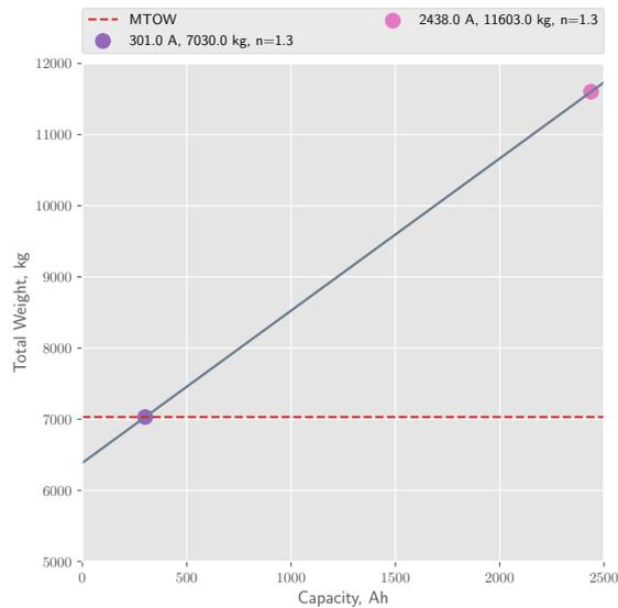
FIGURE 4.6: Effect of increasing battery capacity on weight (21 PAX).
