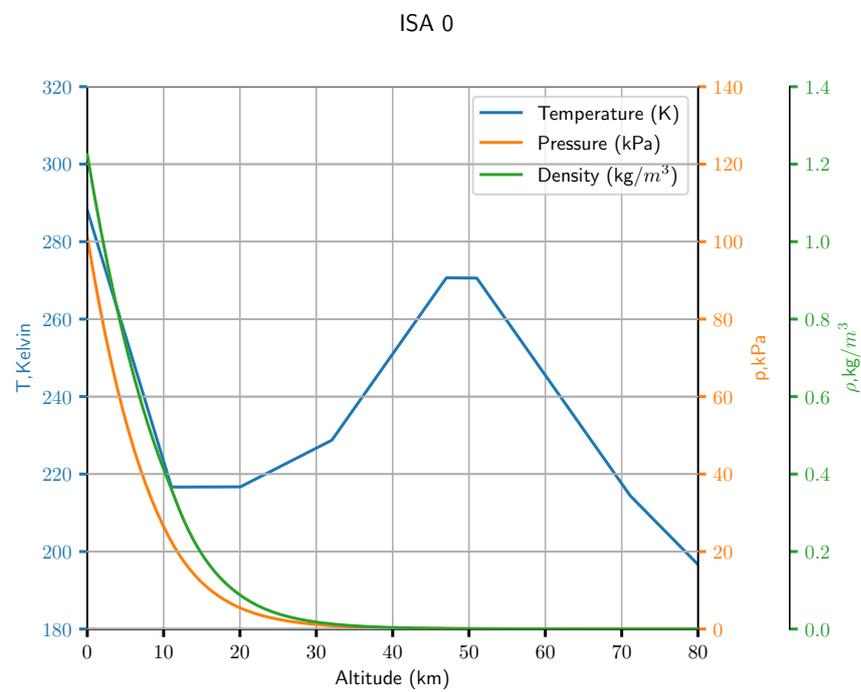
FIGURE 2.1: Variation of pressure, density and temperature In the International Standard Atmosphere
