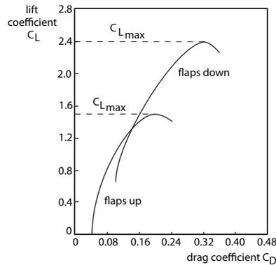
FIGURE 2.10: Lift-drag polar for a low subsonic airplane (estimated) (Ruijgrok, 2009)
