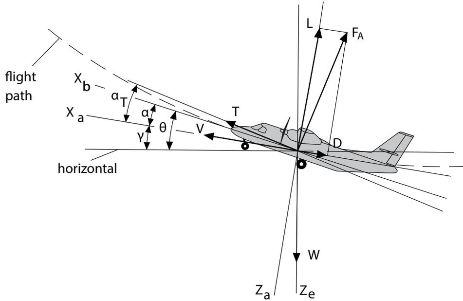
FIGURE 2.34: Airplane In symmetric flight (Ruijgrok, 2009).
