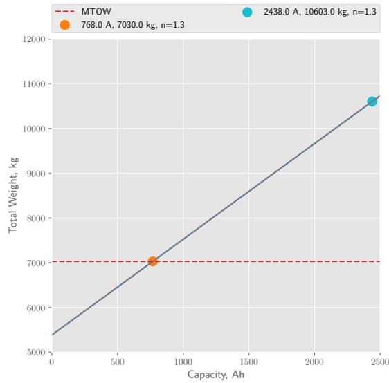
FIGURE 4.5: Effect of increasing battery capacity on weight (11 PAX).
