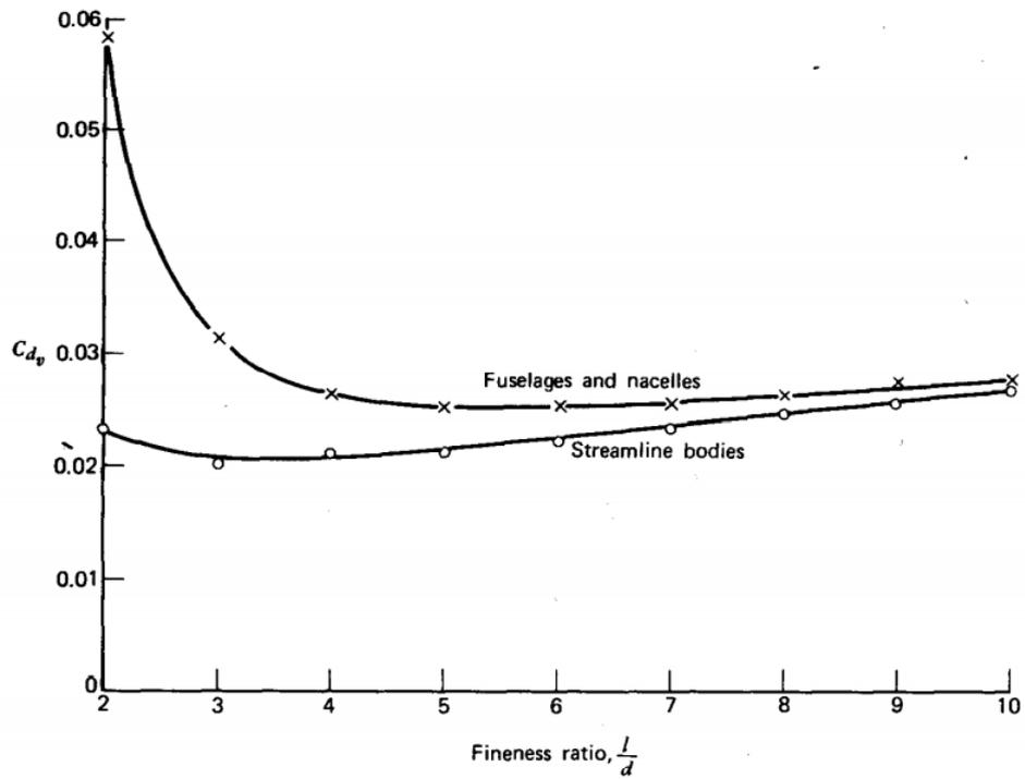
FIGURE 2.24: Drag coefficients based on volume for bodies as a function of fineness ratio. (McCormick, 1994)
