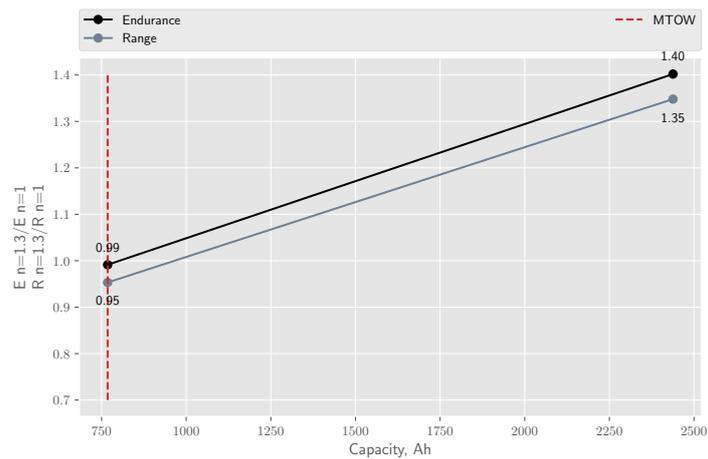
FIGURE 4.3: Effect of battery n-rate (11 PAX).
