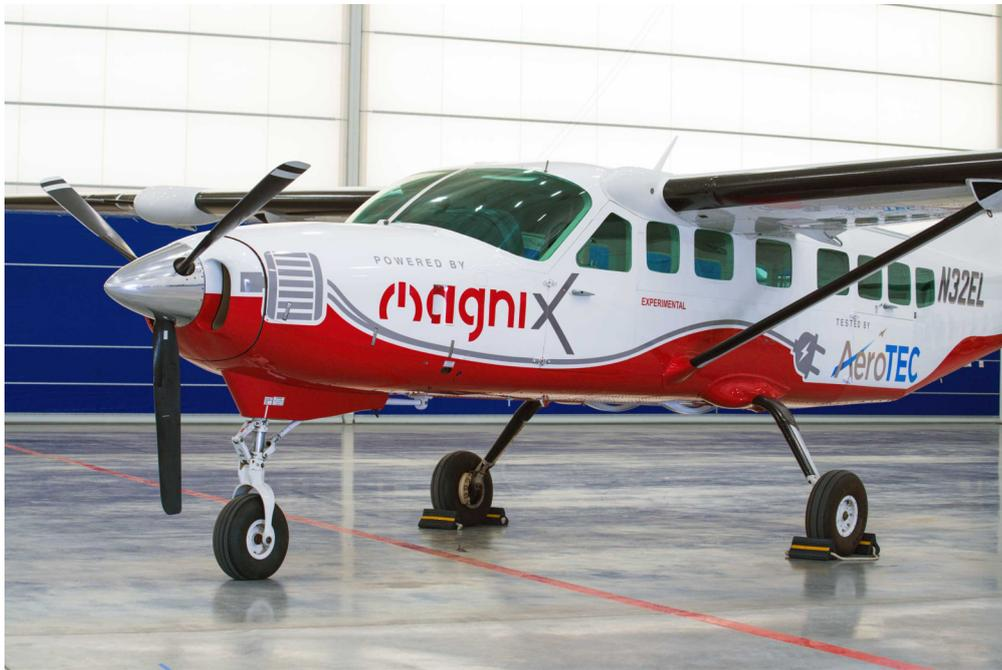
FIGURE 1.4: Cessna B208 eCaravan by magniX and AeroTEC (Calderwood, 2020).
