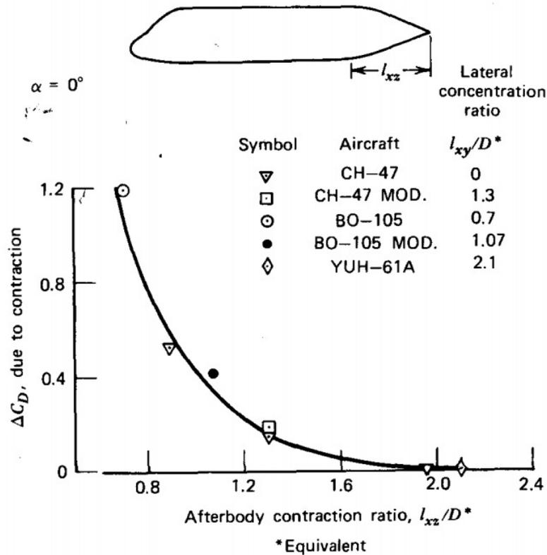
FIGURE 2.25: Effect of afterbody contraction ratio on drag. (McCormick, 1994)
