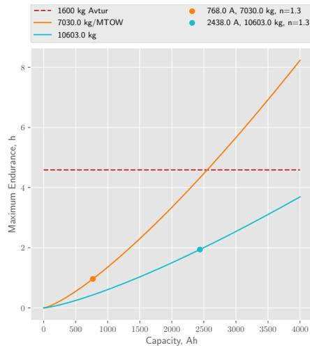
FIGURE 4.9: Effect of increasing battery capacity on maximum endurance (11 PAX).
