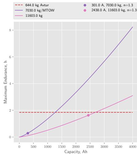
FIGURE 4.10: Effect of increasing battery capacity on maximum endurance (21 PAX).
