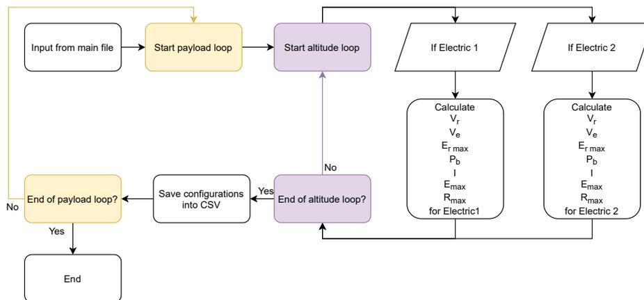
FIGURE 3.14: Maximum electric range and endurance flow chart
