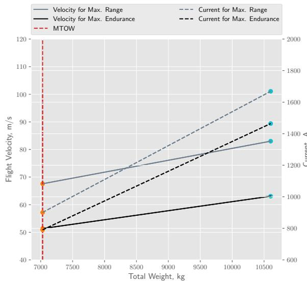
FIGURE 4.7: Effect of increasing total weight on optimum airspeed and currente (11 PAX).
