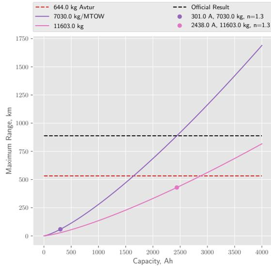
FIGURE 4.12: Effect of increasing battery capacity on maximum range (21 PAX).
