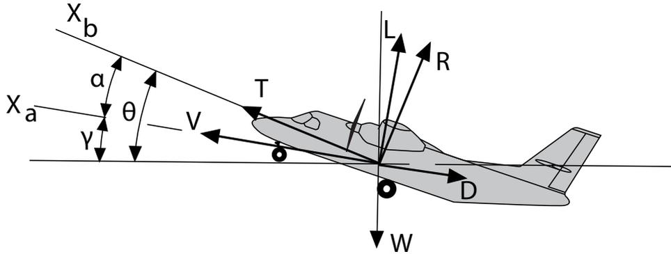
FIGURE 2.2: Free body diagram
