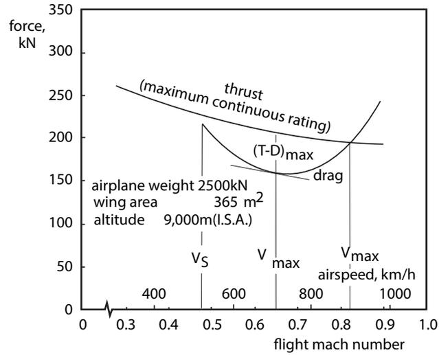
FIGURE 2.38: Performance diagram for turbofan transport airplane (Ruijgrok, 2009).
