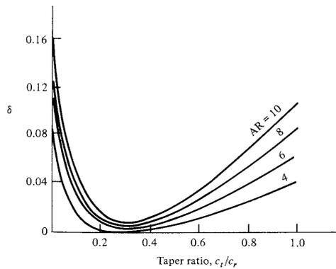
FIGURE 3.5: Induced drag coefficient vs taper ratio.
