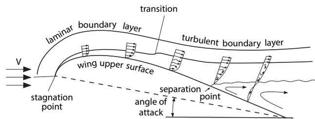
FIGURE 2.13: Development of the boundary layer over the wing (Ruijgrok, 2009)
