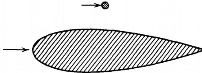
FIGURE 2.26: Two bodies having the same drag (supercritical flow). (McCormick, 1994)
