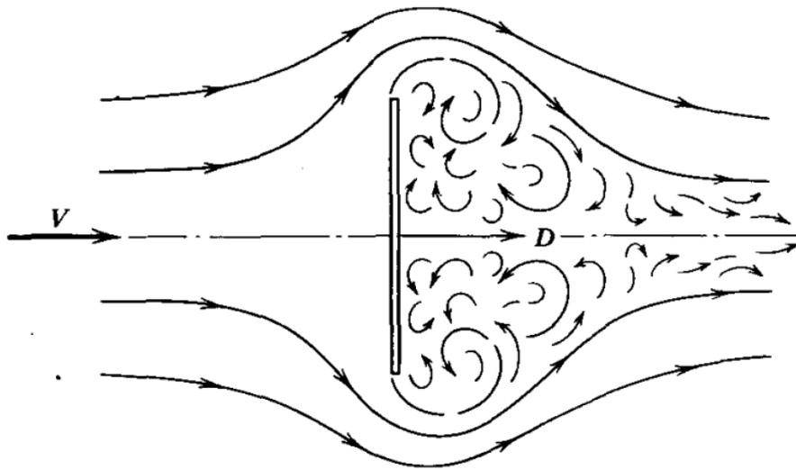
FIGURE 2.16: Flat plate normal to flow (McCormick, 1994)
