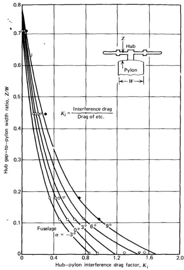
FIGURE 2.28: Effect of hub pylon gap on interference drag. (McCormick, 1994)
