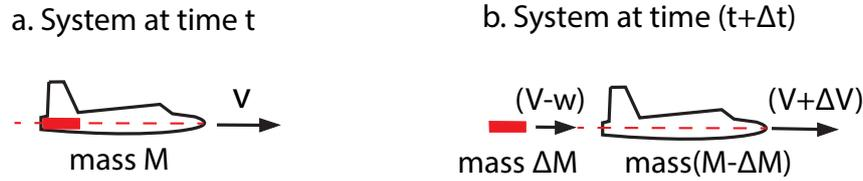
FIGURE 2.3: Ejection of airplane mass (Ruijgrok, 2009)
