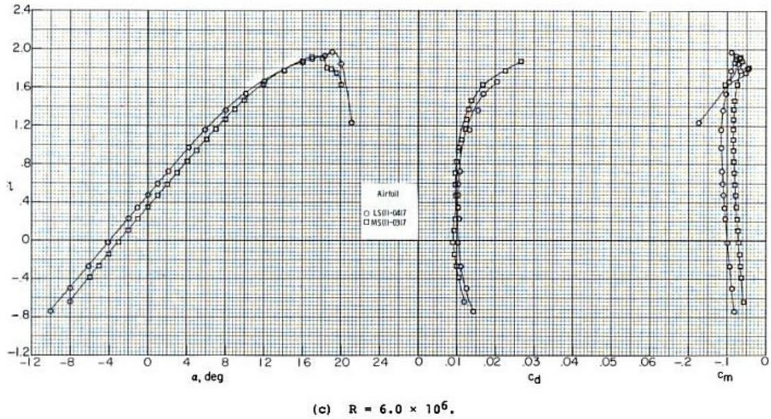
FIGURE 3.3:  $c_l$ ,  $c_d$ , and  $c_m$  at  $Re = 6 \times 10^6$
