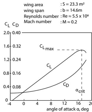
FIGURE 2.9: Aerodynamic characteristics of a low-subsonic airplane (estimated) (Ruijgrok, 2009)
