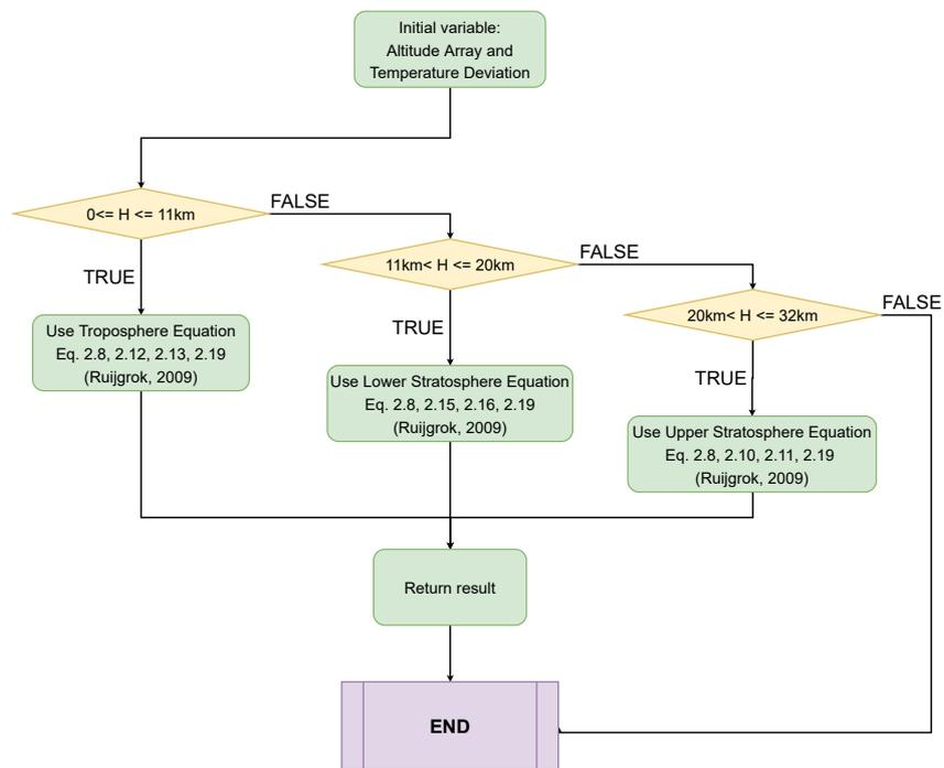
FIGURE 3.9: ISA computational model flow chart (H is geometrical altitude)
