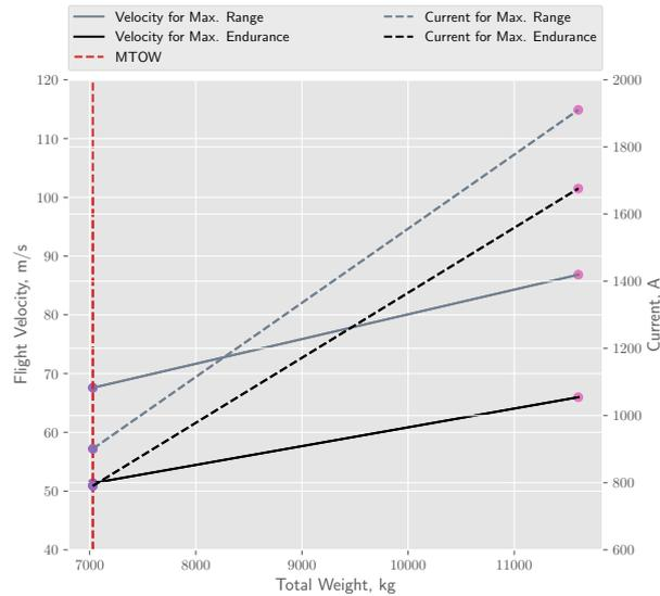
FIGURE 4.8: Effect of increasing total weight on optimum airspeed and current (21 PAX).
