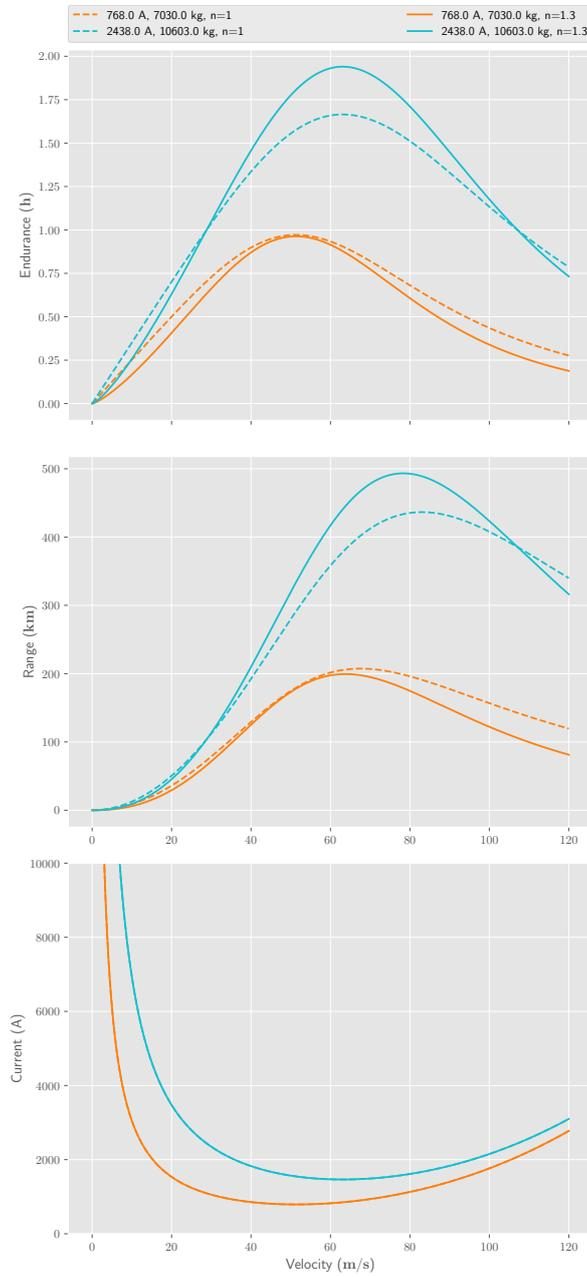
FIGURE 4.1: Range on Endurance based on airspeed 11 PAX (1100 kg payload).
