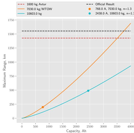
FIGURE 4.11: Effect of increasing battery capacity on maximum range (11 PAX).
