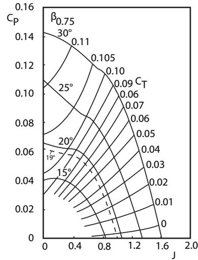
FIGURE 2.37: Propeller chart of 2-bladed propeller (estimated)
