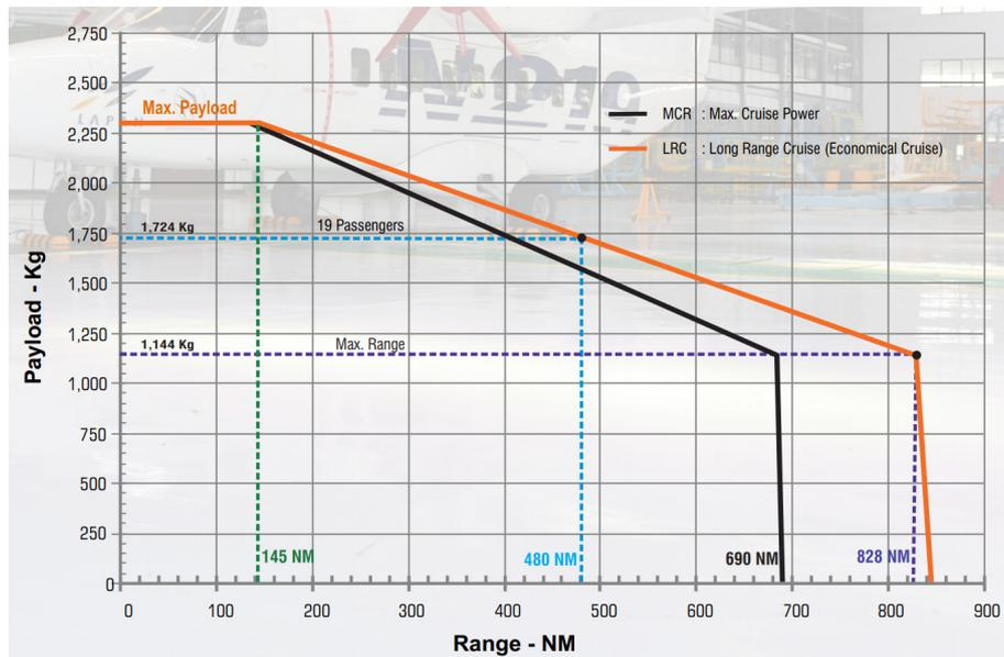
FIGURE 1.8: N-219 Payload Range (*N219 SOLUTION FOR FRONTIER GATEWAY*, 2018).
