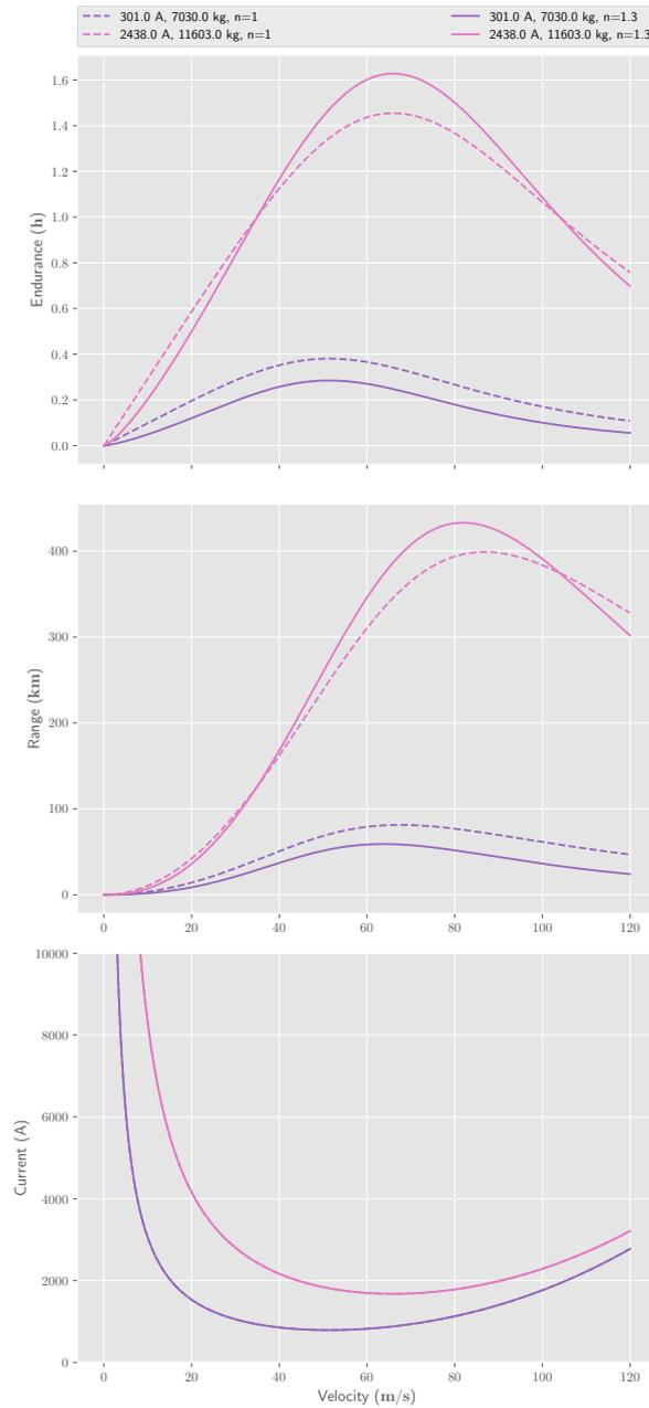
FIGURE 4.2: Range on Endurance based on airspeed 21 PAX (2100 kg payload).
