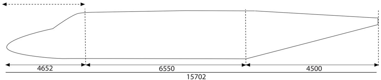
FIGURE 3.6: N-219 fuselage estimation
