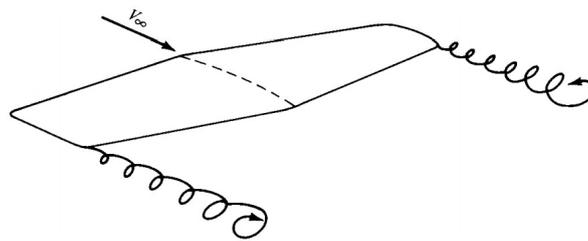
FIGURE 2.32: Schematic of wing-tip vortices (Anderson, n.d.).
