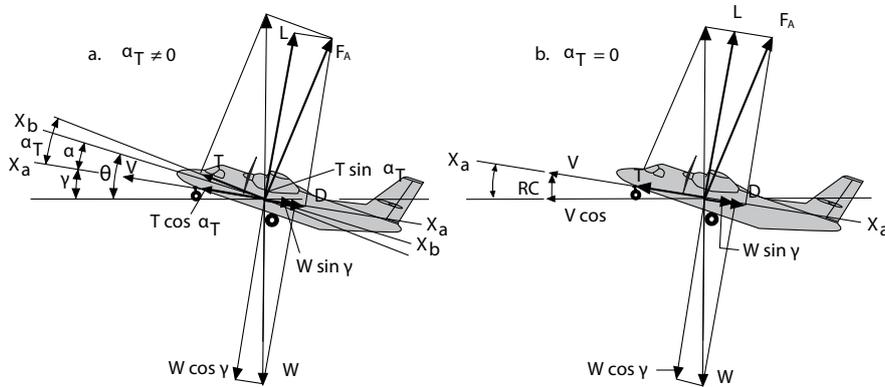
FIGURE 2.35: Airplane In steady symmetric flight (Ruijgrok, 2009).
