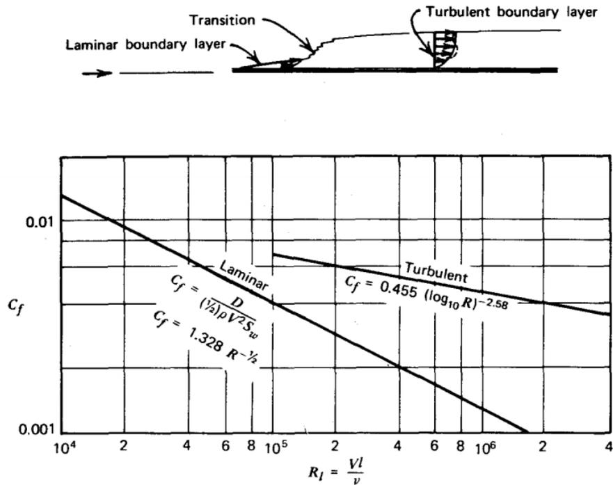
FIGURE 2.15: Drag of a thin flat plate (McCormick, 1994)
