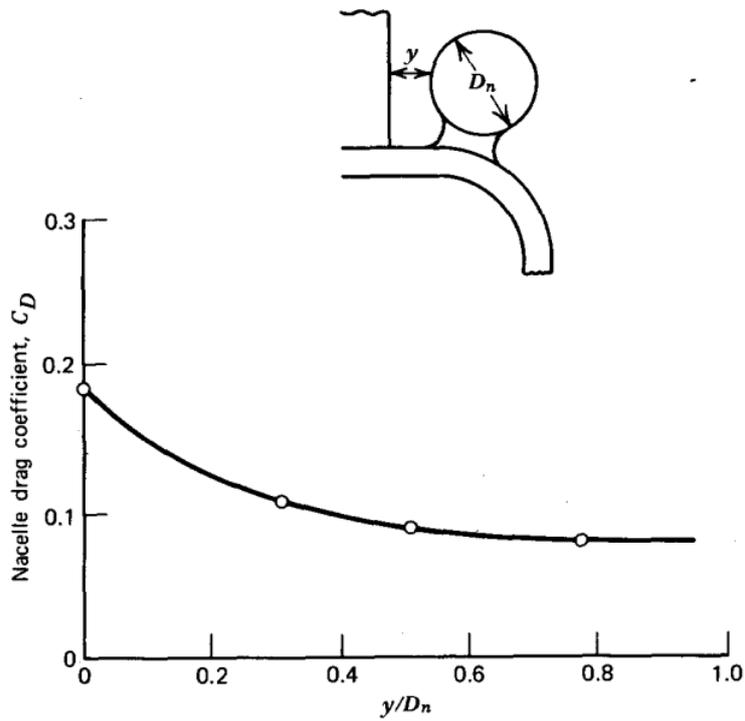
FIGURE 2.27: Effect of nacelle location on interference drag. (McCormick, 1994)
