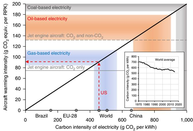
FIGURE 1.1: Warming intensity of a projected first-generation all-electric aircraft and of a current-generation jet engine aircraft versus carbon intensity of electricity. (Schäfer et al., 2019).
