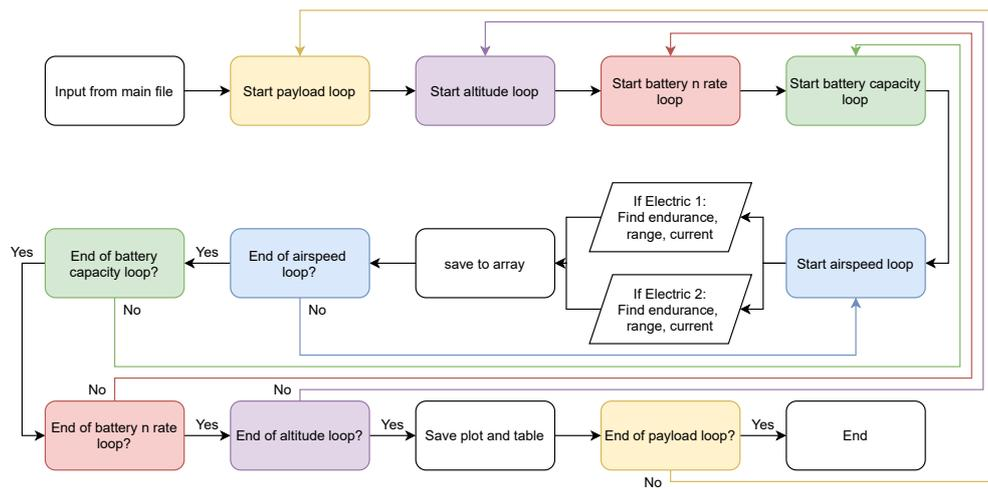
FIGURE 3.12: Electric range, endurance, and current relation flow chart
