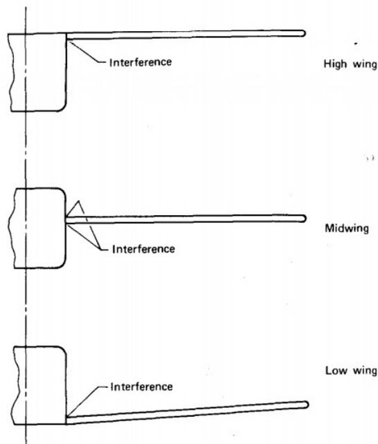
FIGURE 2.29: Wing-fuselage interference drag. (McCormick, 1994)
