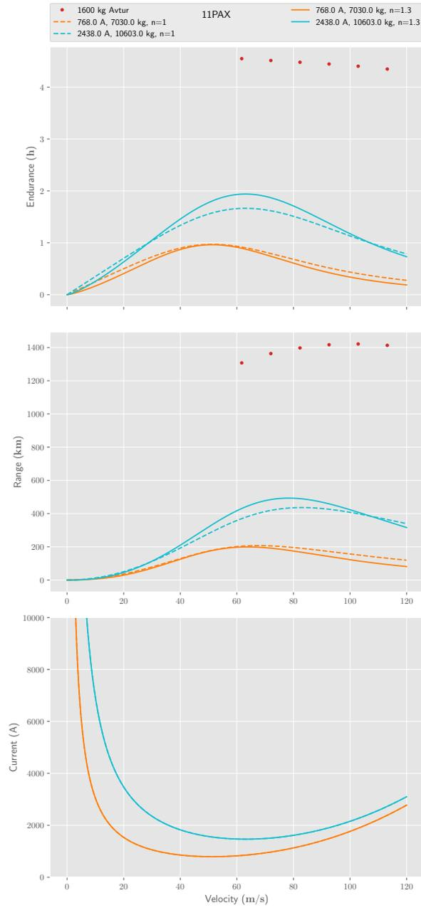
FIGURE 4.13: Electric and airbreathing N-219 comparison (11 PAX).
