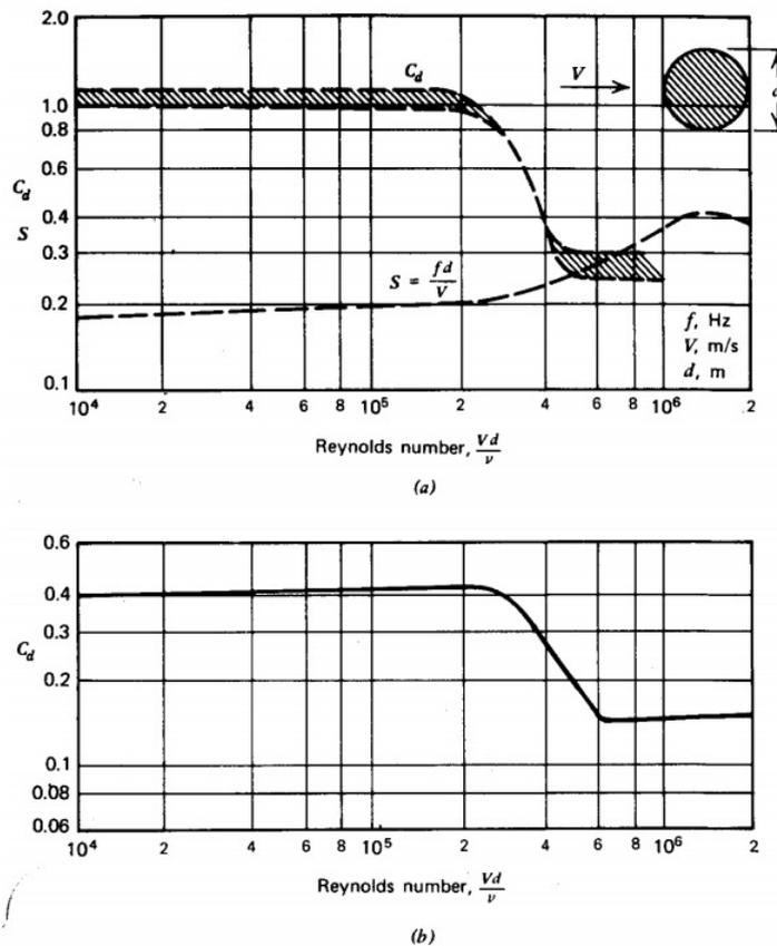
FIGURE 2.19: Drag coefficients of cylinders and spheres vs Reynolds number. (a) Two-dimensional circular cylinder. (b) Spheres. (McCormick, 1994)
