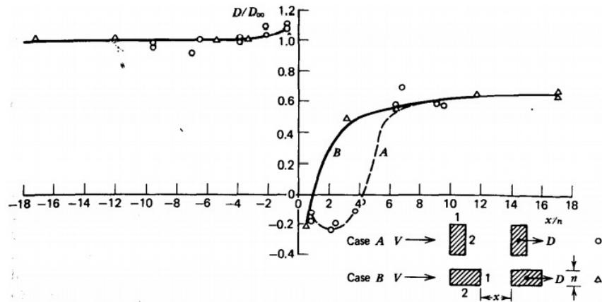
FIGURE 2.30: Interference drag for a two-dimensional rectangular cylinder in tandem with another. (McCormick, 1994)
