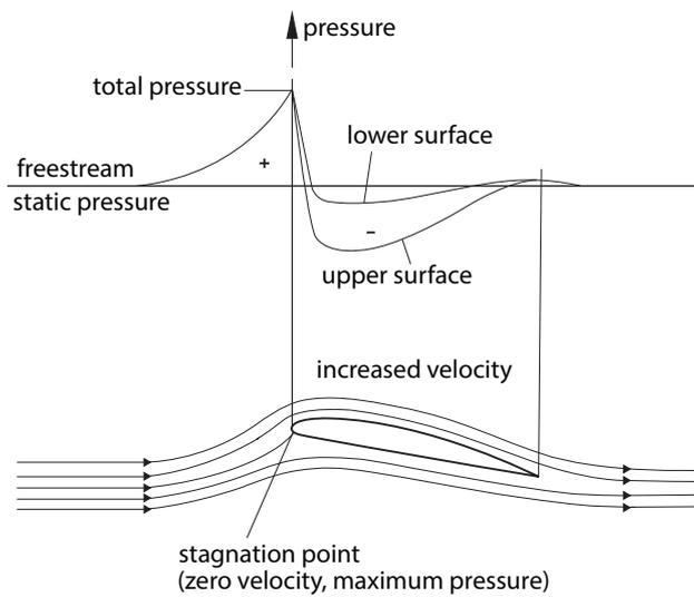
FIGURE 2.4: Pressure distribution over a wing section (Ruijgrok, 2009)
