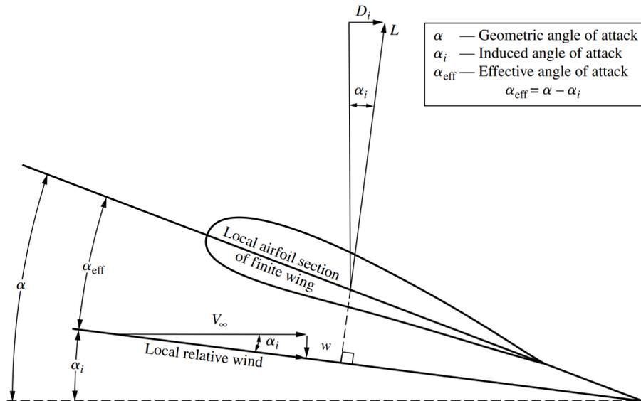
FIGURE 2.33: Effect of downwash on the local flow over a local airfoil section of a finite wing (Anderson, n.d.).
