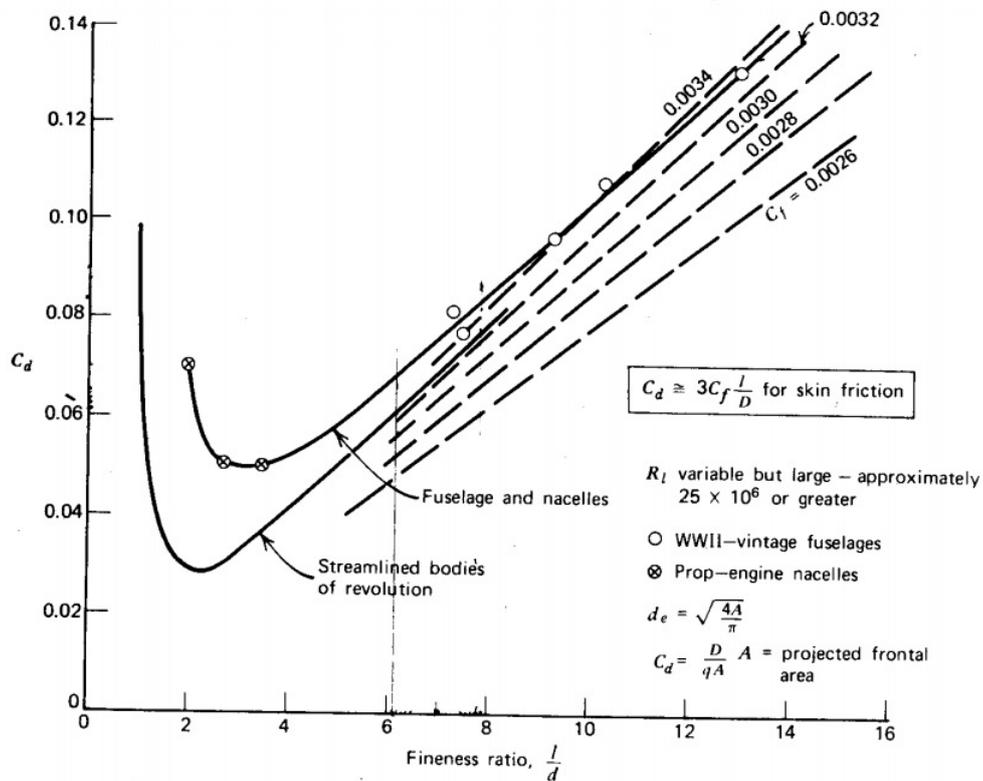
FIGURE 2.23: Drag of fuselages and similar shapes. (McCormick, 1994)
