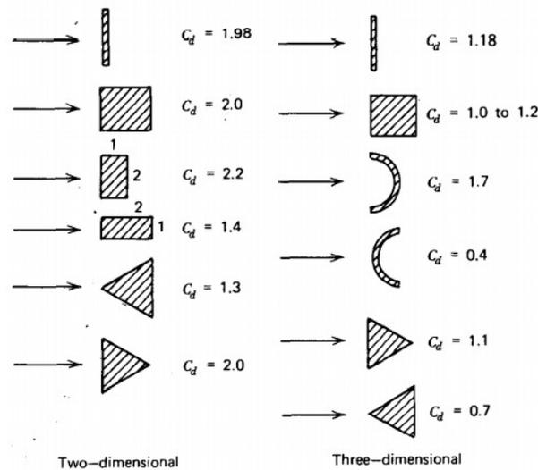
FIGURE 2.20: Examples of shapes having Cd values nearly independent of Reynolds number. (McCormick, 1994)
