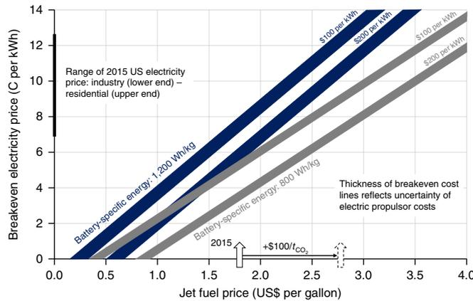
FIGURE 1.2: Break-even electricity price for a first-generation all-electric aircraft. (Schäfer et al., 2019).
