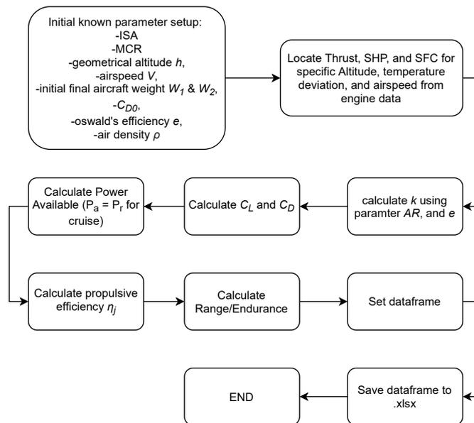
FIGURE 3.10: Range and endurance airbreathing aircraft flow chart table
