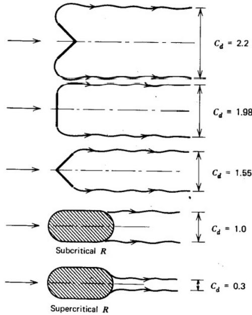
FIGURE 2.22: Qualitative estimate of drag for two-dimensional shapes. (McCormick, 1994)
