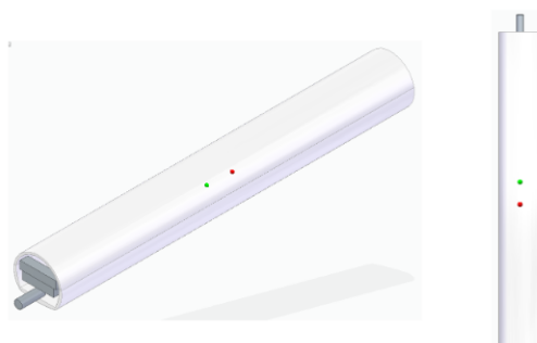
FIGURE 4.13: Enclosed Fuselage with Center of Mass in Green dot and Center of Volume in Red dot (Source: Personal Documents)
