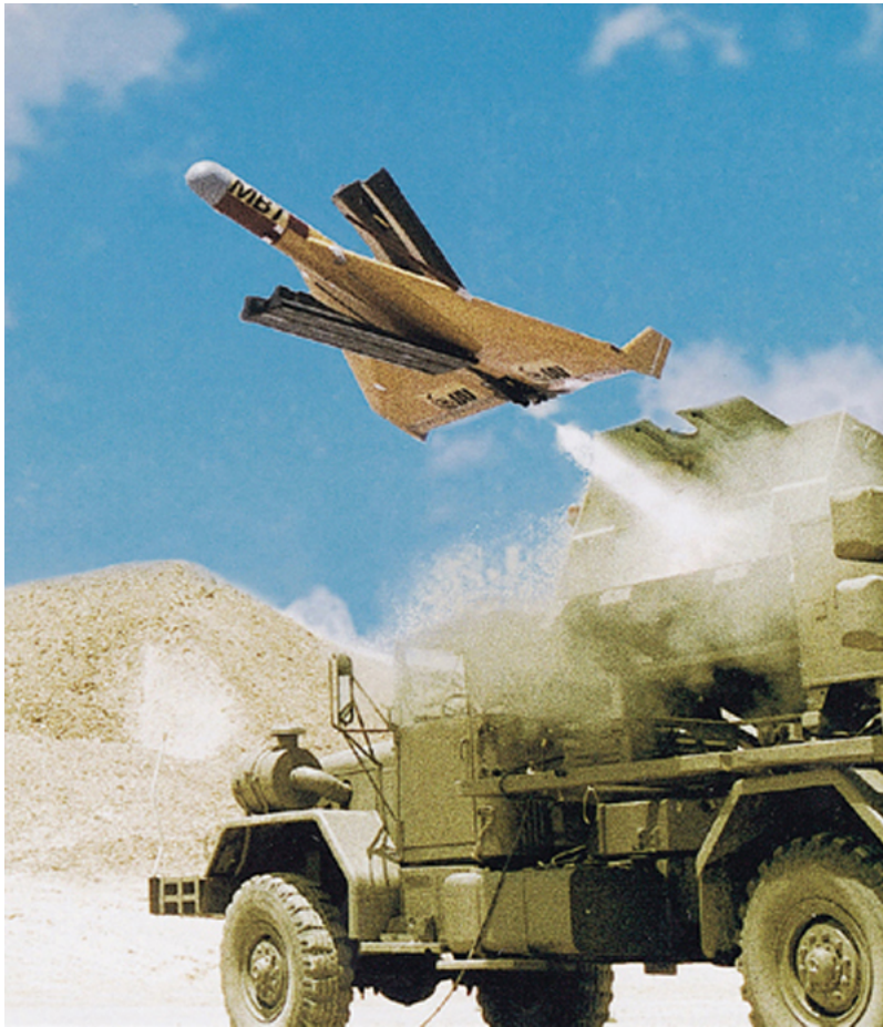
FIGURE 4.68: Cold or Hot Canister launch, shown by IAI Harpy launching.
