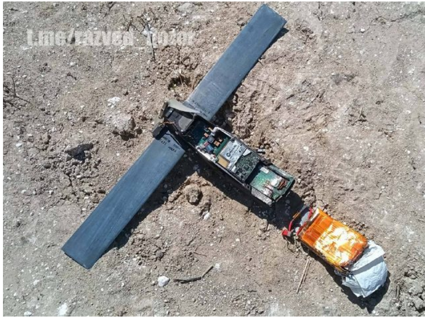
FIGURE 4.64: Aerovironment Switchblade 300 after committed self-destruct.
