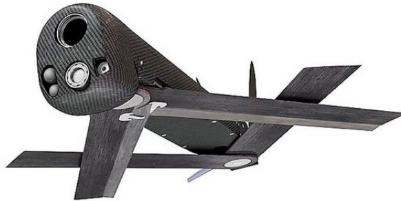
FIGURE 4.1: One of the best benchmarks in Loitering Munitions against infantry or light vehicles, AeroVironment Switchblade 300
