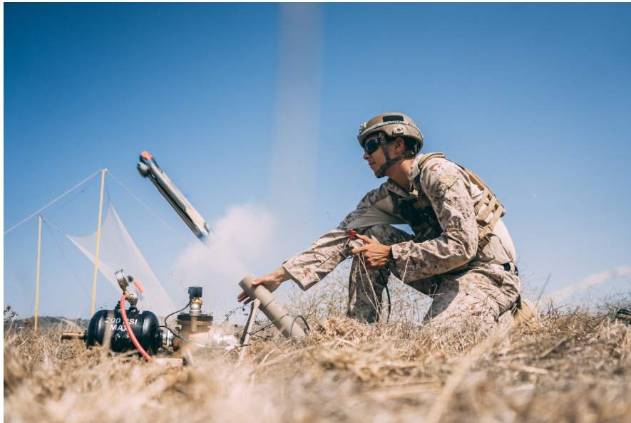
FIGURE 4.70: AeroVironment Switchblade 300 launched in gas pressurized tube.
