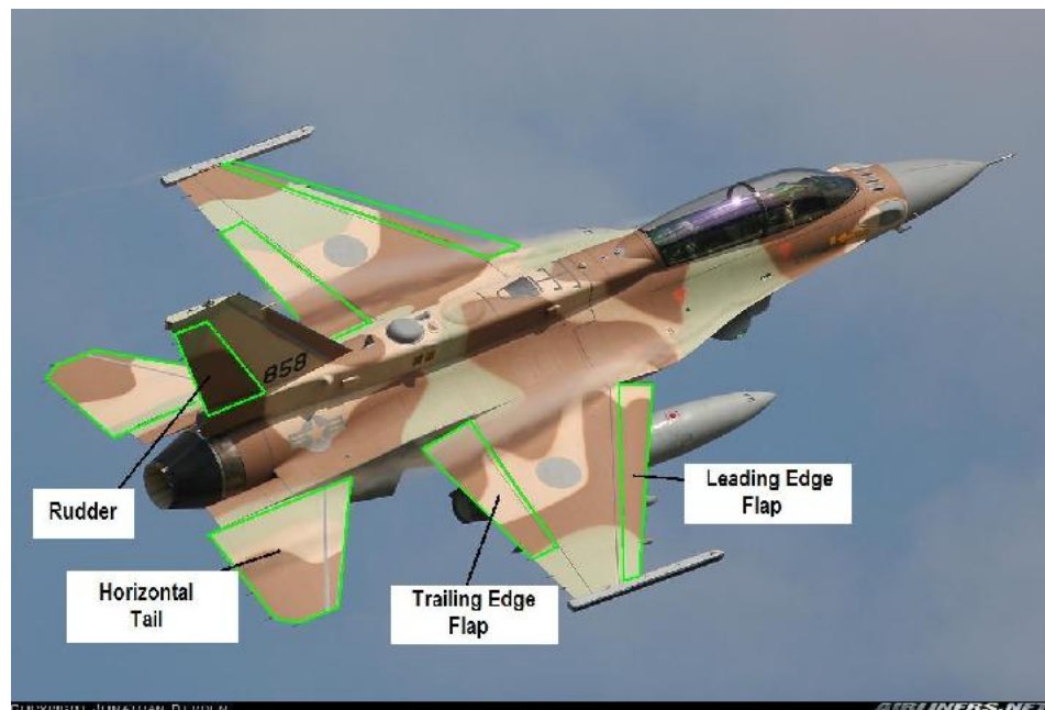
FIGURE 4.66: F-16 Fighting Falcon's Control Surface diagram, includes Flaperons and Elevons/Tailerons
