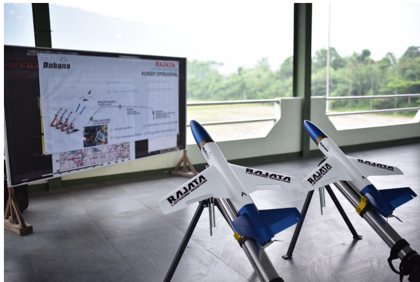
FIGURE 4.71: Dahana RAJATA with the gas pressurized rails.
