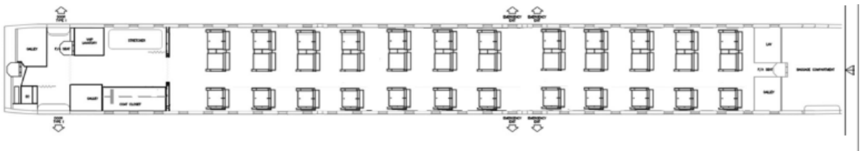
FIGURE 4.2: Second option of proposed business jet configuration.
