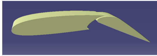
Figure 3.4: Illustration of Fowler flap [11].
